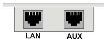
Figure 4 RJ45 Ports on IP Flush/OR Master Stations
