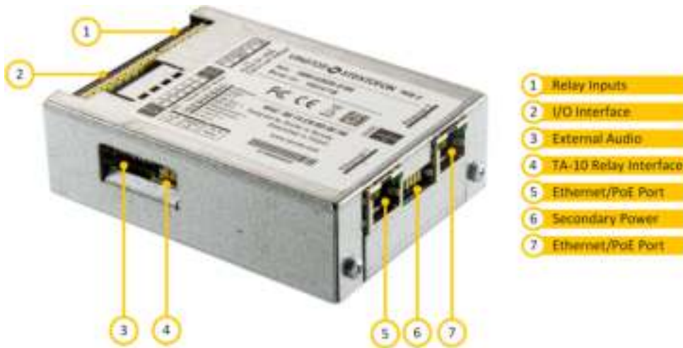
Figure 8 TKIE-2 Connectors & Functions
