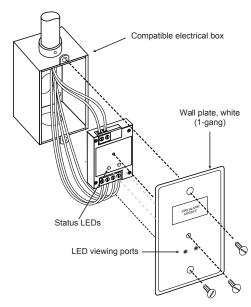
**SIGA-MCT2:** mount the UIO motherboard inside a suitable ED-WARDS enclosure with screws and washers provided. Plug the SIGA-MCT2 into any available position on the motherboard and secure the module to the motherboard with the captive screws. Wiring connections are made to the terminals on the motherboard (see wiring diagram). UIO motherboard terminals are suited for #12 to #18 AWG (2.5 mm² to 0.75 mm²) wire size.
