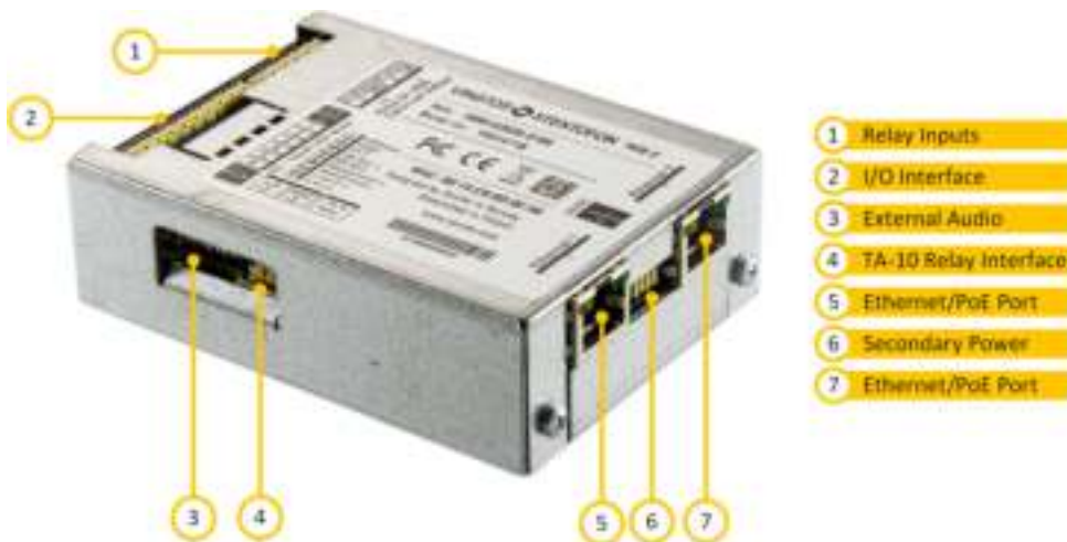
Figure 8 TKIE-2 Connectors & Functions
