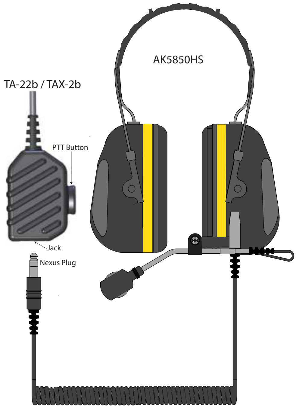
Figure 13 AK5850HS Headset with TA-22b/TAX-2b Plugbox
