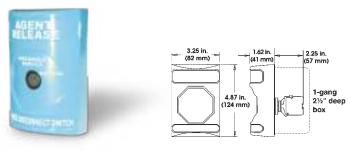
The service disconnect switch is used to temporarily disable the fire suppression system. One switch is installed on each of the two release circuits between the SIGA-REL and the RELA-EOL end-of-line relay. Opening the Service Disconnect Switch allows the fire alarm system to be tested without activating the fire suppression system. The operation of this switch causes a trouble signal at the control panel.
