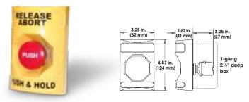
The abort station is a normally-open, non-latching device. It is used to prevent the release of agent into the protected area after the release sequence has begun.
