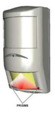
If the lens is masked, a photodiode receives reduced IR energy levels. The detector then sends a trouble signal to the security system indicating that someone masked the detector.
