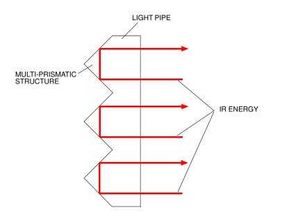
When the prismatic structure is coated with a spray material, the reflective properties of the prisms are negated, allowing the IR energy to pass through the prisms and out of the detector.
