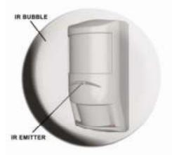
If the detector is blocked, an above-normal level of IR energy reflects back through the detector's lenses. The detector uses multiple IR photodiodes to detect the extra IR energy levels, then sends a trouble signal to the security system indicating that someone masked the detector.
