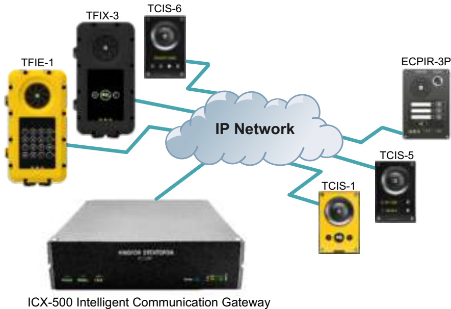
Figure 14 ICX-AlphaCom Intercom System
